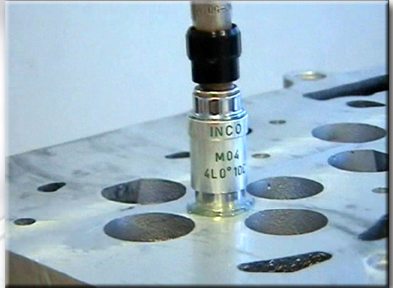
Sensor over the area, where chamber was suspected
