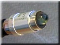
The ultrasound sensor with water based jelly
